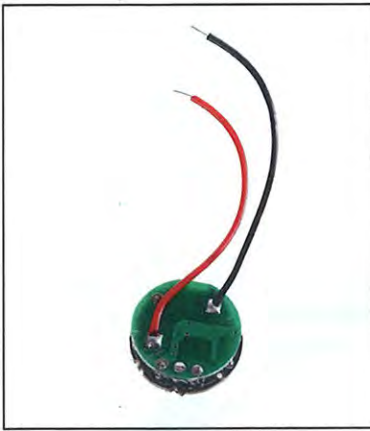
3V~8.4V 5W Cree 5-Mode Memory Circuit Board for Flashlights (16.7mm*6.3mm) $2.99
